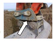
There are three main quick hitch systems on the market; manual, automatic & semi-automatic. Employers or users of this equipment must be familiar with the safe operation and use of the relevant type.
